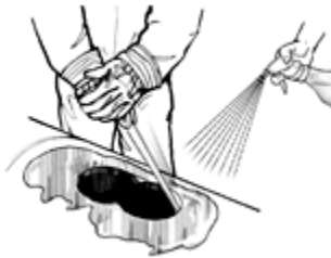
Hand Sawing Asbestos Cement Pipe
